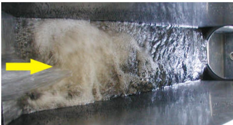
Figure 8: Filter DN 300,  $Q_{300,F} = 7,4 \text{ l/s}$  (waterlevel reaches the height of the outlet)
