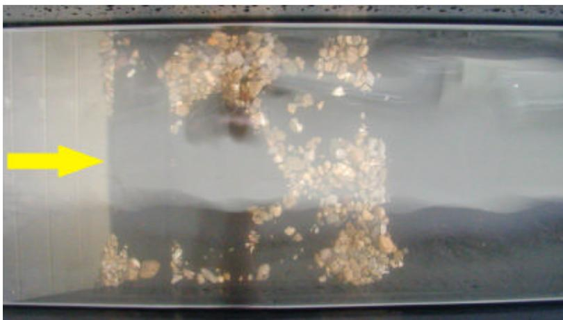
Figure 5: Filter DN 150, after 30 Seconds with flow of  $Q=9,0 \text{ l/s}$  the filter is extensively cleaned (from 3,5 kg stone-sand-composite 150g are remaining)
