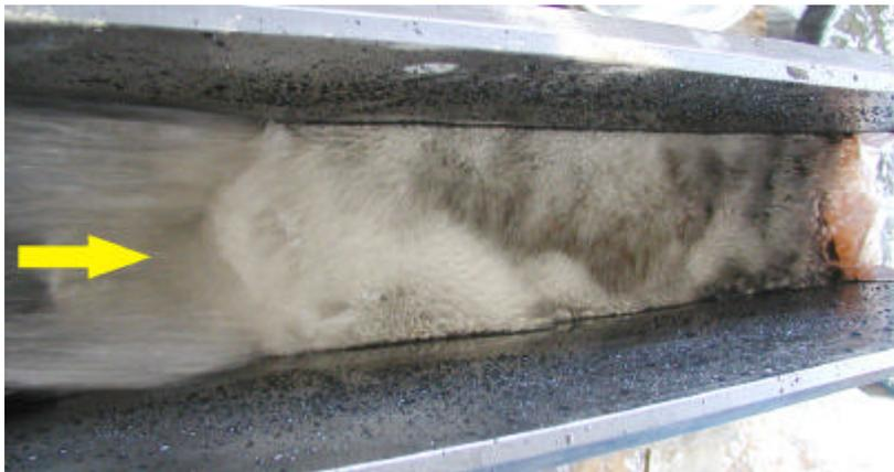
Figure 4: Filter DN 150,  $Q_{150,F} = 6,0 \text{ l/s}$  (hydraulic jump is active, the first stones are rinsed out)
