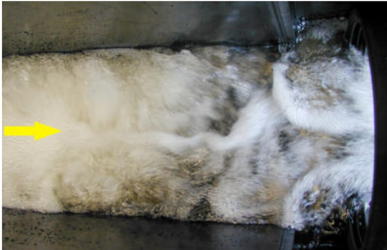
Figure 9: Filter DN 300,  $Q = 18,0$  l/s, very strong hydraulic jump in the filter chassis
