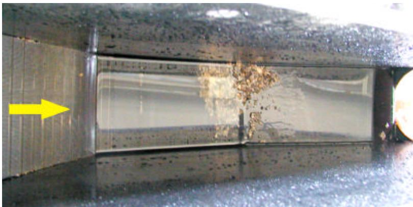
Figure 7: Filter DN 200, after 30 seconds with a flow of  $Q = 11,0 \text{ l/s}$  the filter is extensively cleaned (from 3,5 kg stone-sand-composite 300g are remaining)
