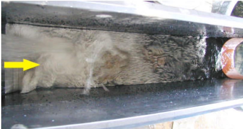
Figure 3: Filter DN 100,  $Q_{150,F} = 2,7 \text{ l/s}$  (waterlevel reaches the height of the outlet)
