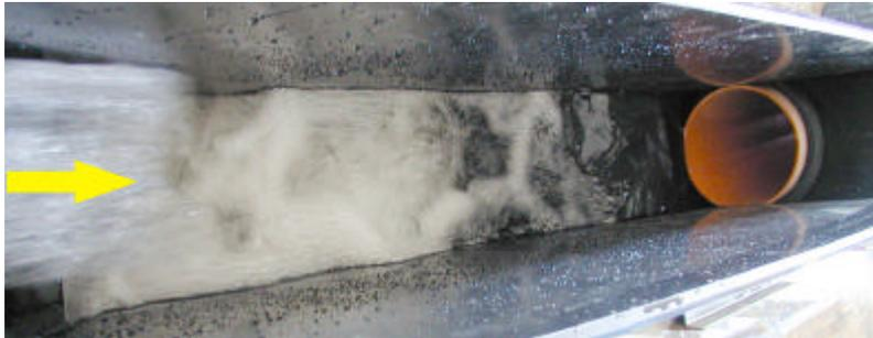
Figure 6: Filter DN 200,  $Q_{200,F} = 5,5 \text{ l/s}$  (waterlevel reaches the height of the outlet)
