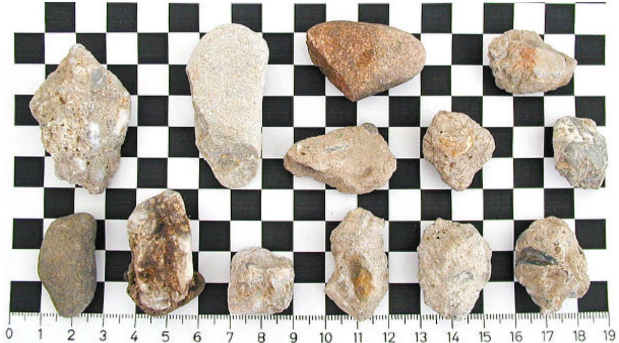
Figure 2: Size of the biggest stones of the sand-stones-composit for the contamination of the INTEWA hydraulic jump filter(Rasterweite 1,0 cm)
