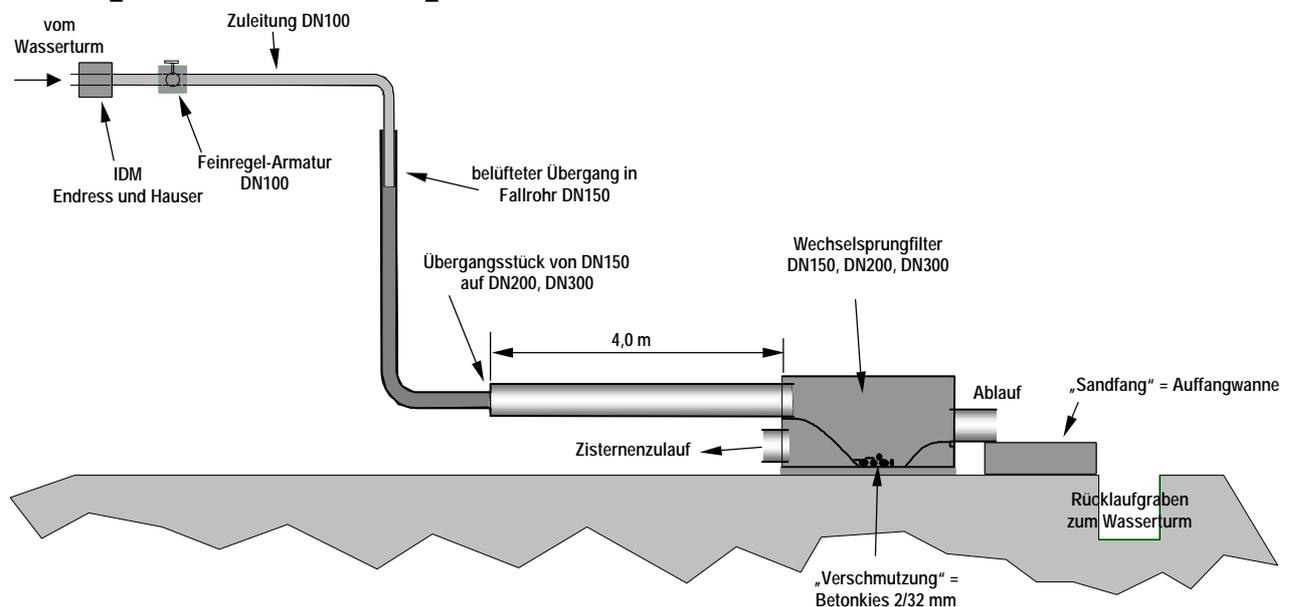
Figure 1: Experimental setup for the acceptance test of the INTEWA hydraulic jump filter
